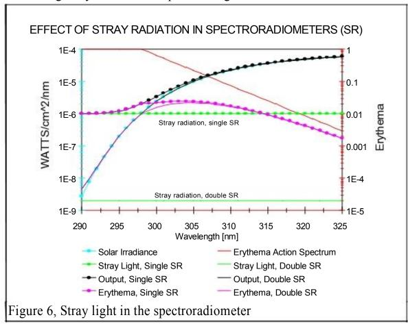
The radiometer also has weak unwanted, or stray radiation. This radiation adds to the total but is of no significance for even low sun where its total contribution is below 1.0
