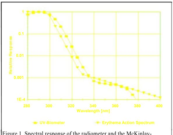
Figure 1. Spectral response of the radiometer and the McKinlay-Diffey erythema action spectrum
